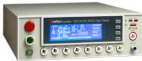
Figure 1.0: Guardian 1000 Series Hipot Tester
